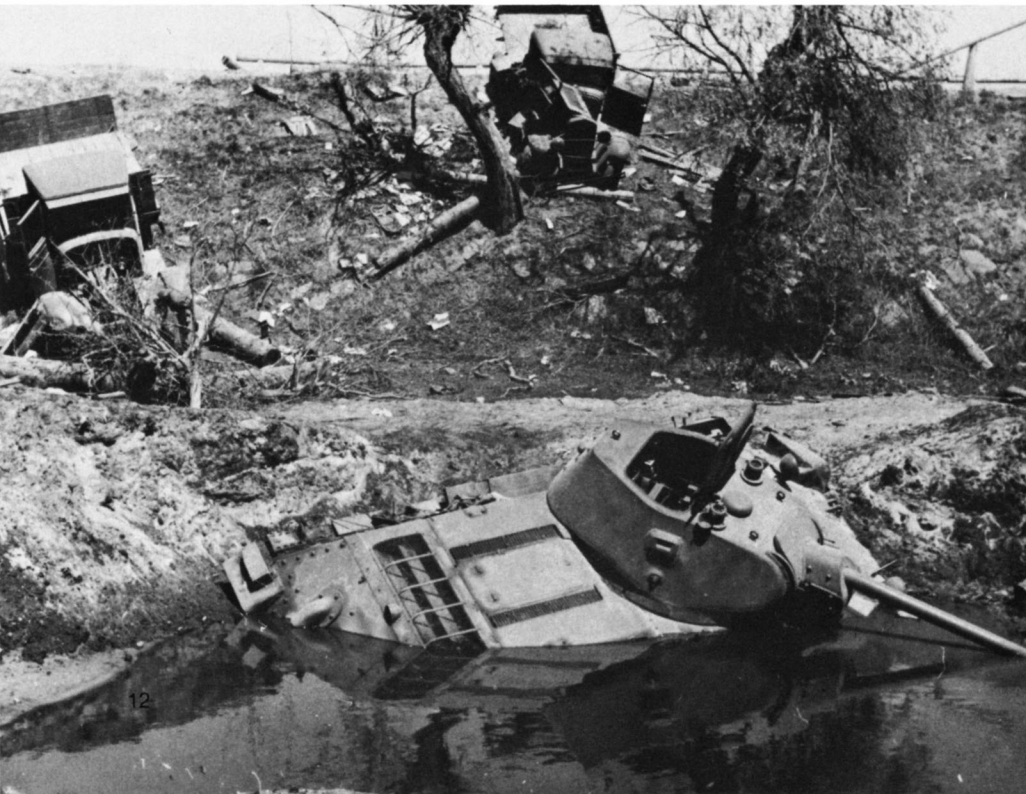
(Above Left) The new T-34 Model 1941 was manufactured with either a cast or welded turret. As on the Model 1940, the cast turret was 52mm thick. This is one of the earliest cast turreted Model 1941s produced, which was knocked out in the opening days of Barbarossa. It still has the panniers fitted. (National Archives)
