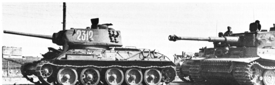
(Below) As the production of the D-5T armed T-34-85s was drawing to a close, some, like this machine, were manufactured with features characteristic of the later Model 1944 like the use of the MK-4 periscope in place of the PTK-5 and the fitting of the radio in the turret instead of the hull. This particular T-34-85 has been knocked out and its gun is jammed at full recoil. It is being passed by a Tiger I of Sch. Panzer Abteilung 505 in 1944. (Bundesarchiv)
