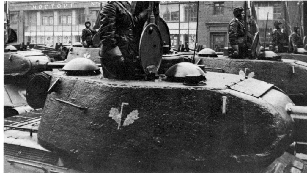
This closeup of the turret of a late war T-34-85 with the 'composite'-style turret was taken in November 1945. It shows the separate dome vents later used on the T-34-85. Note also that the later style one piece hatch is in use. The rough, almost porous appearing surface texture of the armor was particularly evident on machines from this factory. This insignia is that of the 4th Guards Tank Corps. (Sovfoto)
