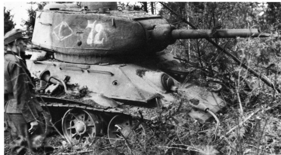
(Below) As the production of the D-5T armed T-34-85s was drawing to a close, some, like this machine, were manufactured with features characteristic of the later Model 1944 like the use of the MK-4 periscope in place of the PTK-5 and the fitting of the radio in the turret instead of the hull. This particular T-34-85 has been knocked out and its gun is jammed at full recoil. It is being passed by a Tiger I of Sch. Panzer Abteilung 505 in 1944. (Bundesarchiv)
