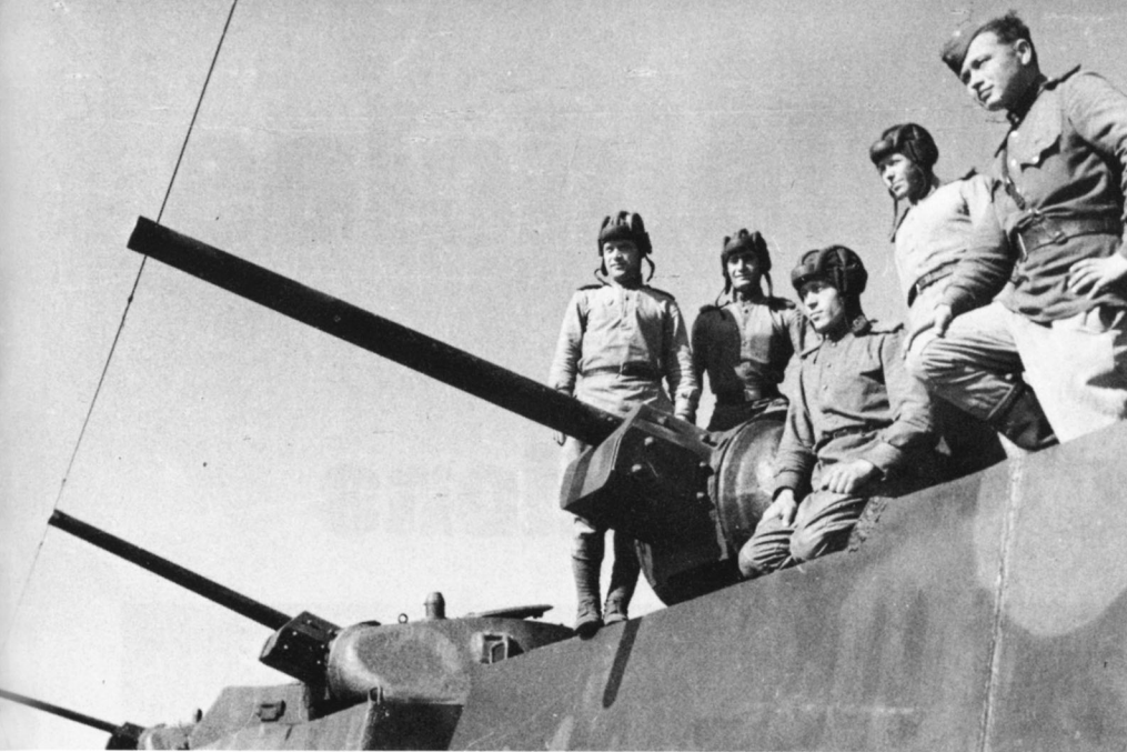
One of the off shoots of the T-34 was the tank-turreted armored train, bronepoyezd , used to provide mobile artillery fire and to protect trains. This particular one, the famous Ilya Mourametz , saw action from the first year of the war and, in this photo, is seen while engaged in shelling outside of Warsaw in August 1944. It used T-34 Model 42 turrets. Others used turrets from the Model 1941, T-26, T-28, T-35 or KV heavy tanks. (Sovfoto)
