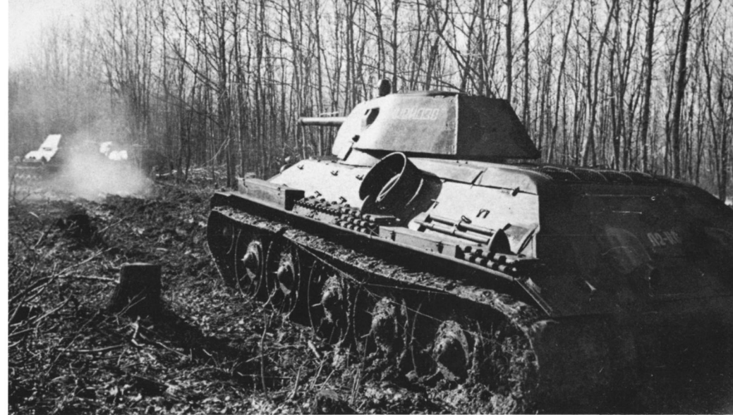
The T-34 Model 1941s produced at STZ with welded turrets had simplified turret rears with a flat rear plate like the one seen here from the South West Front in April 1942. The large circular object on the hull side is an extra brake lining for the transmission. This vehicle was named Ordzhonikidze after the Soviet leader and has the script L2-IS on the rear access panel. (Sovfoto)
