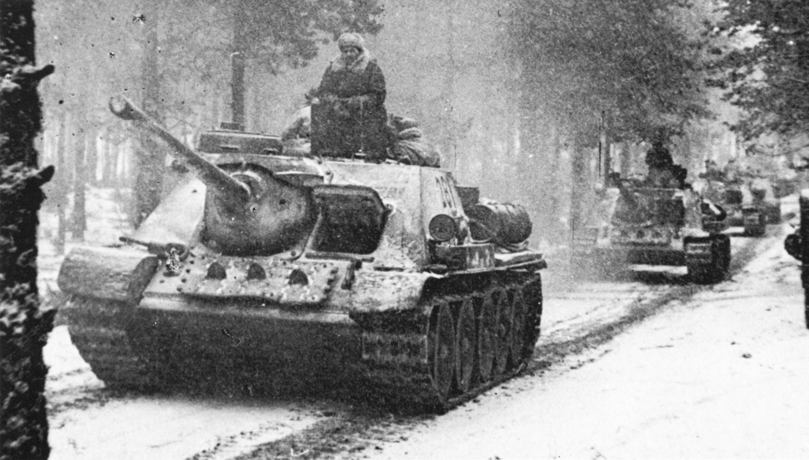
A column of new SU-100s move through a fog shrouded wood in East Prussia in January 1945. The SU-100 can be distinguished from the similar SU-85 by the larger gun, the commander's cupola on the right of the vehicle roof and double dome ventilators. (Sovfoto)
