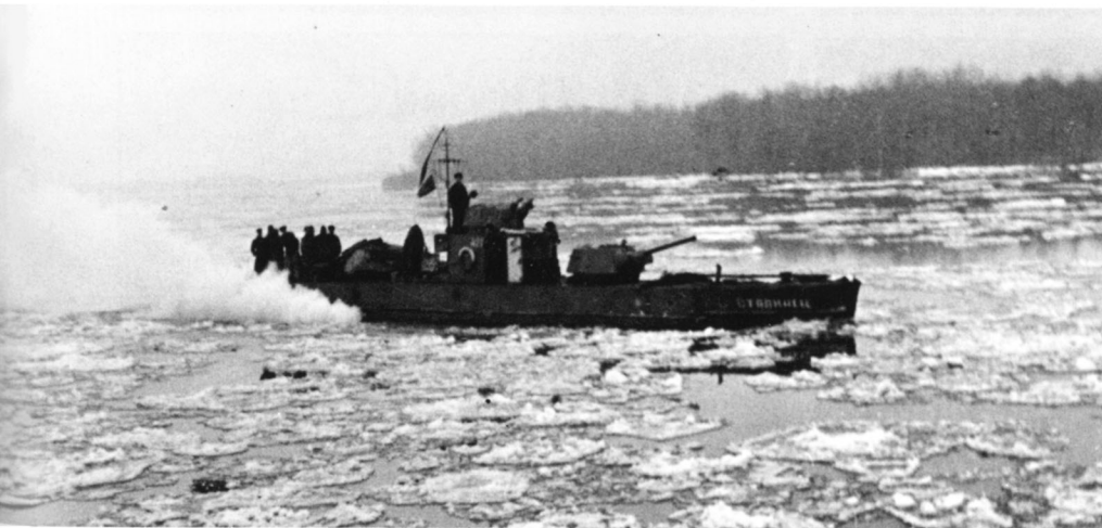
Surprisingly, large numbers of T-34 turrets were used on Type 1124 armored river gunboats, like this one, Stalinetz , of the Danube River Flotilla. This gunboat has a T-34 Model 43 turret fore and aft as well as a small machine gun turret amidships. They were used to patrol along contested river routes and to provide fire support. This particular monitor was photographed during the battle for Budapest. (Sovfoto)
