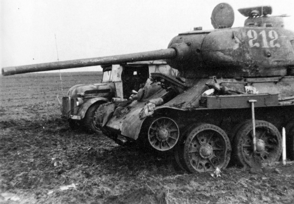
This T-34-85 Model 1944 of the 'flattened' turret type uses the common, spoked, rubber-rimmed roadwheel. The early split hatch on the turret cupola is visible. (Bundesarchiv)
