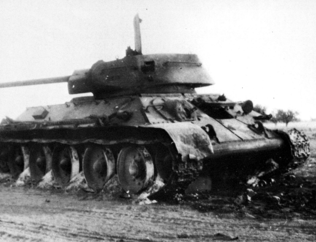
A T-34 Model 42 of the Polish 2 pulk czołgow (1 Tank Regiment) moves forward near Sielce in July 1943. Note the early style fuel boxes.
