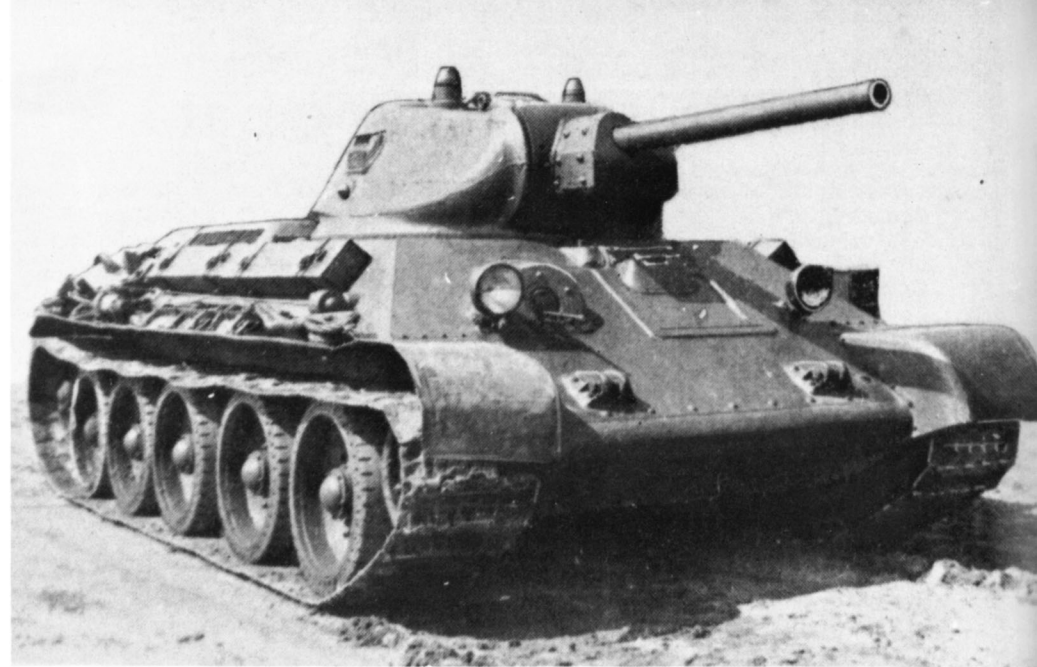
This is a stock shot of a freshly manufactured T-34 Model 1941 (cast turret, commander's vehicle) with full stowage and fittings. It is unusual in that it is fitted with the later style waffle pattern track.
