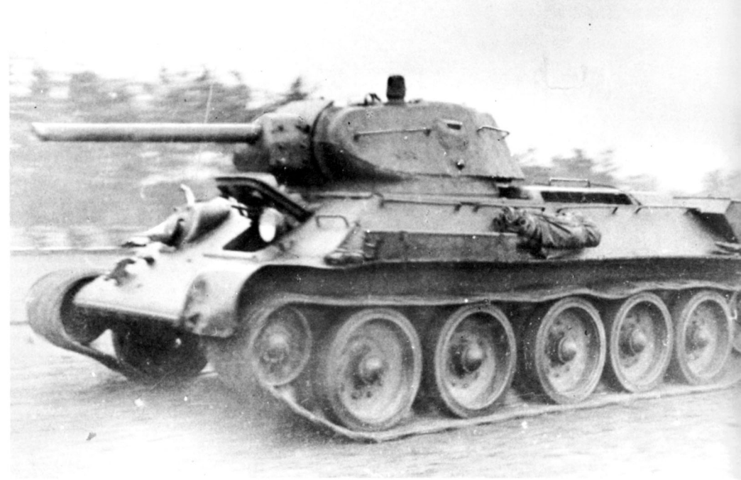
A T-34 Model 42 of the Polish 2 pulk czołgow (1 Tank Regiment) moves forward near Sielce in July 1943. Note the early style fuel boxes.
