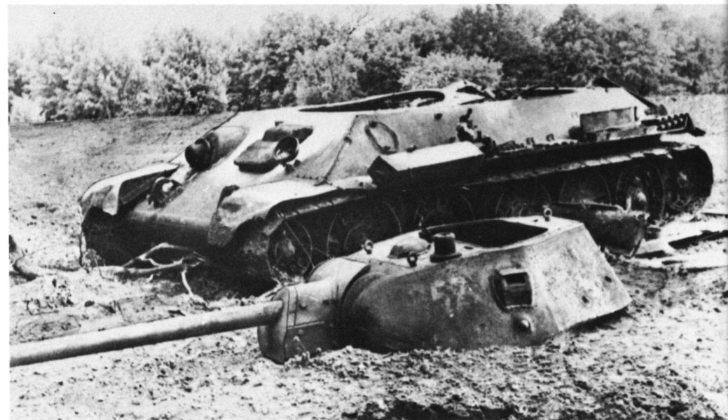
The fuel container in this OT-34 exploded, blowing off the turret. This OT-34 is based on a T-34 Model 1942 and the flame projector mantlet is clearly visible in place of the machine gun.
