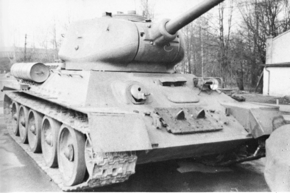
The Czechoslovak-manufactured T-34-85 was the most numerous of the foreign-produced derivatives. The turret casting differed in small details and in contour, but was basically similar to the Soviet style. (Charles Kliment)
