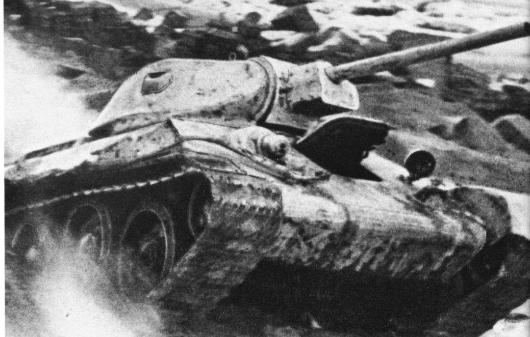
The pudgy mantlet of the ATO-41 distinguishes this OT-34 as a flamethrower tank. These vehicles stowed their fuel internally and were otherwise identical to regular gun tanks. The flamethrower replaced the hull machine gun.
