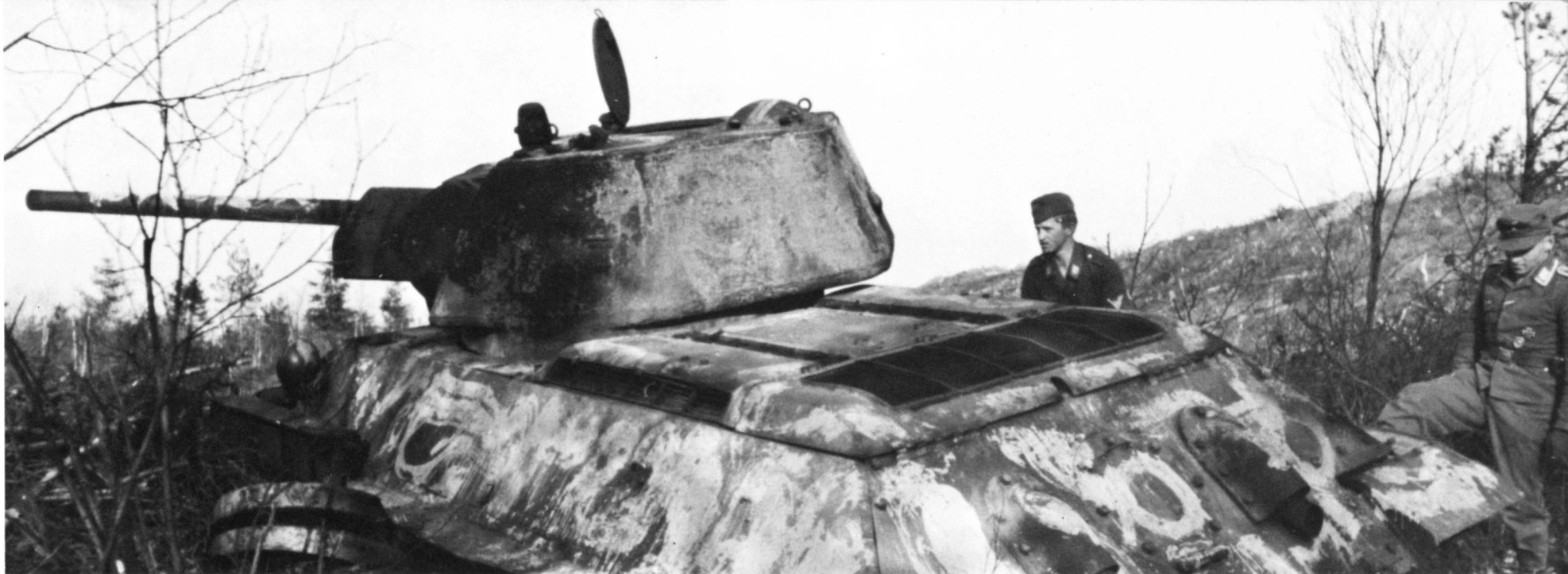
This early production T-34 Model 43 with 'softedge' turret has very few exterior fittings and carries a rather unusual swirl-style camouflage paint finish. It was disabled in a bog, winter 1942. (Bundesarchiv)
