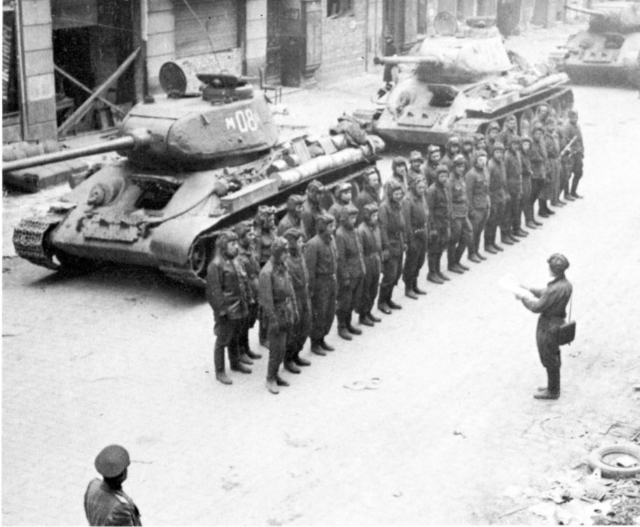
A Soviet tank company is briefed in the outskirts of Berlin before the final drive. The T-34-85s are of the later 'composite' turret style and lack the pronounced flattening at the turret sides which was characteristic of those produced at other factories. (Sovfoto)
