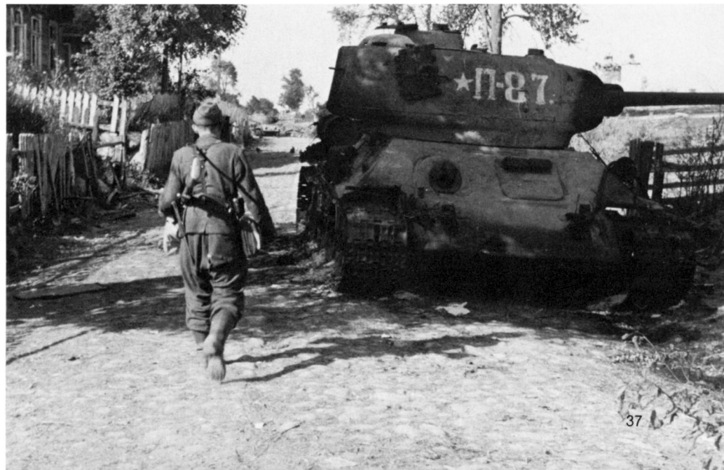
This T-34-85 Model 1944 of the 'flattened' turret type uses the common, spoked, rubber-rimmed roadwheel. The early split hatch on the turret cupola is visible. (Bundesarchiv)
