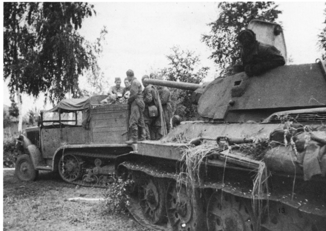
This STZ-manufactured T-34 Model 1941 has just captured a German Citroen-Kegresse halftrack. The T-34 is fitted with the all steel roadwheels and is using the special, wide 550mm track for improved handling on soft ground and snow. (Sovfoto)
