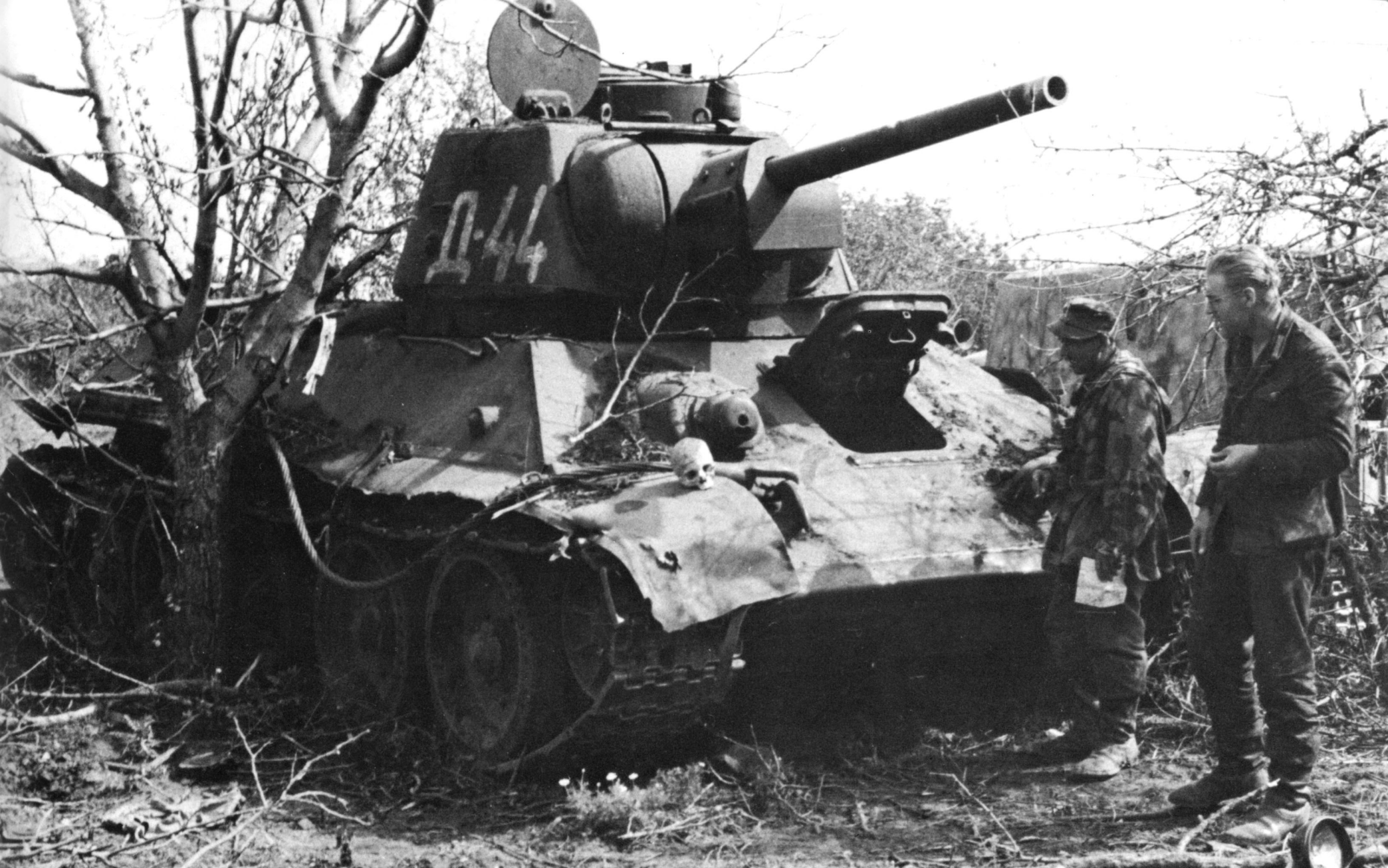
This knocked-out OT-34 is based on the chassis of a late-production T-34 Model 43 with a '85 style pointed nose. The turret number is D-44. Note that the radio hull mount is plugged over due to the transfer of the radio to the turret. The skull, possibly that of a crew-member, is a token of the great price paid by the Russians in the 'Great Patriotic War'. (Bundesarchiv)
