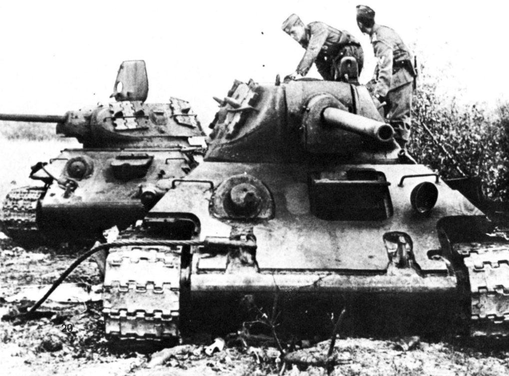
German troops examine a pair of disabled T-34 Model 42s from Zavod Nr. 112 . The vehicle in the foreground has very thick added armor, probably as much as 35mm.
